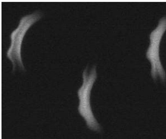
FIGURE 3. Droplets of 50 \text{ mg ml}^{-1} bovine serum albumine (BSA) visualized with calcein fluorescent dye, along the bumpy serpentine channel, with flow rates of 3 \mu\text{l min}^{-1} for the oil stream and 0.3 \mu\text{l min}^{-1} for the BSA streams.
